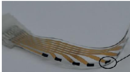
Medtronic 5-6-5 spinal cord stimulation paddle \sim 0.06 \text{ cm}^2 GSA
